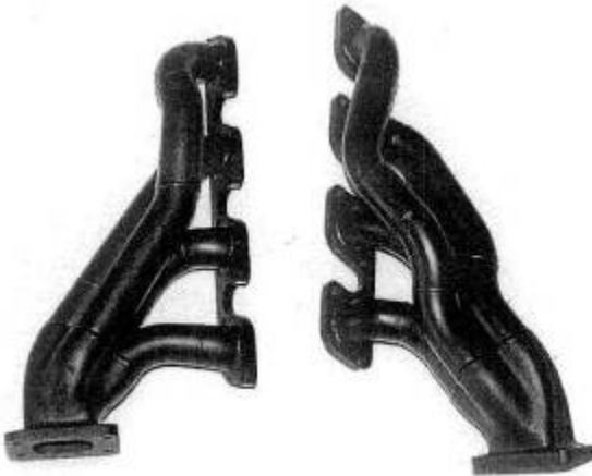
Fig. 10-5. Four-into-one designs for 4- or 8-cylinder engines
