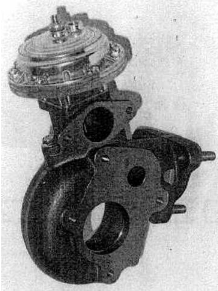
Fig. 12-13. A variation on the integral wastegate, but with a separate vent path
