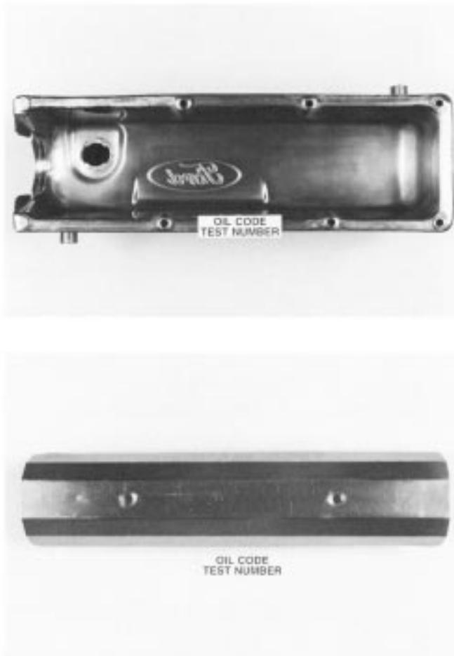
FIG. A7.14 Rocker Arm Cover and Camshaft Baffle Photographs
