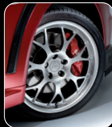
19" 'Stelvio' › forged alloy wheel Wheel and tyre package (1 pce) SR012048
