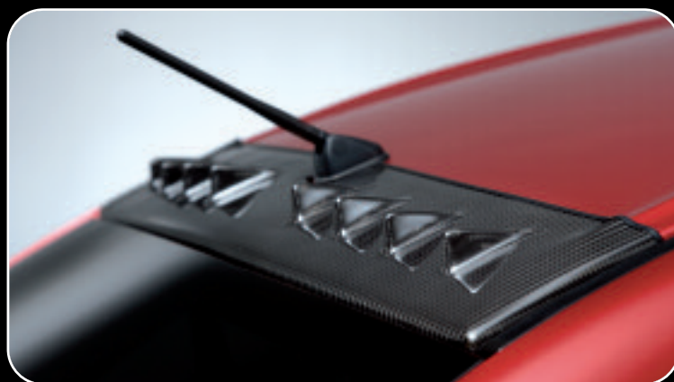
Vortex generator › Carbon fibre. (Standard on FQ-360 models.) SR012065
