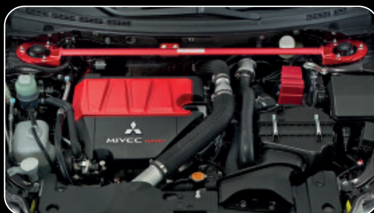
Front strut bar Aluminium replacement strut bar with Lancer Evolution badge. Saves 1.7kg of weight. MZ568879EX
