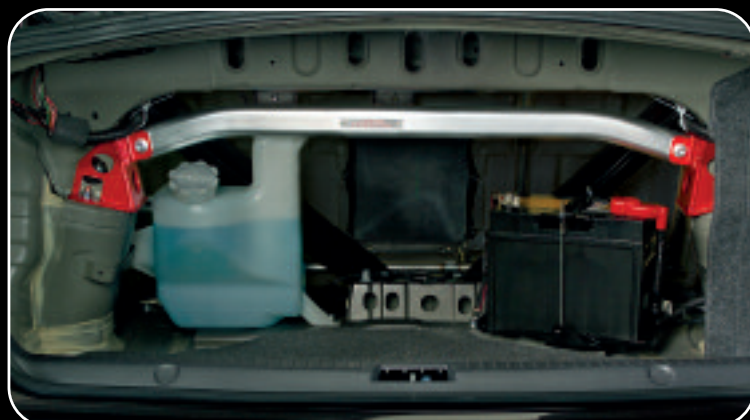
Rear strut bar › Aluminium to increase rear body stiffness. With Lancer Evolution badge. MZ574598EX
