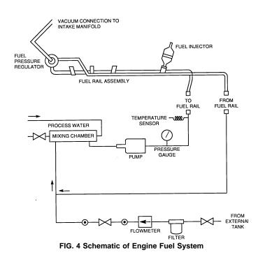
initial boiling point of Phillips J<sup>25</sup> fuel. To ensure good atomization of the fuel, maintain the fuel pressure above 27 psig (186 kPa). In addition, the fuel pressure should be constant at all steady-state conditions to ensure good speed, power, and air-fuel ratio control.
