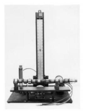
FIG. A3.33 Typical Camshaft Lobe Flow Rating Apparatus
