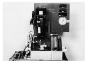
FIG. A3.31 Oil Pump Calibration Apparatus
