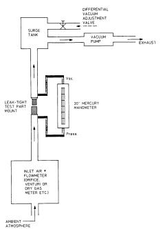
FIG. A3.34 PCV Valve Flow Test Apparatus
