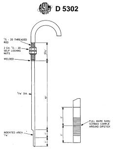
FIG. A3.28 Typical Adjustable Dipstick Fabrication
