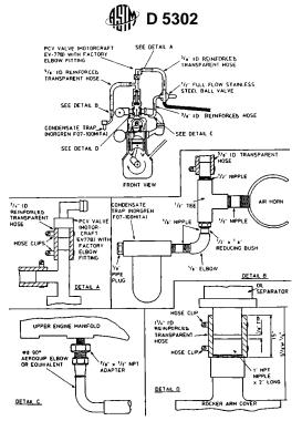
FIG. A3.15 Closed Crankcase Ventilation System, Required Fittings and Parts Configuration
