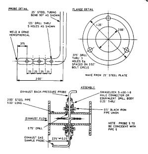
NOTE 1—Bend external tubing segment after assembly parallel with probe axis as shown. This permits visual alignment check during operation.
