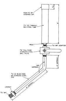
FIG. A3.27 Typical Crankcase Oil Fill Tube and Cap
