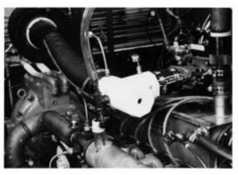
FIG. A3.3 Intake Air Supply System, Air Horn
