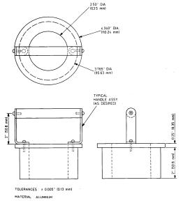
FIG. A3.37 Piston Ring Positioner
