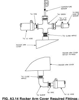
FIG. A3.14 Rocker Arm Cover Required Fittings and Sensor Locations
