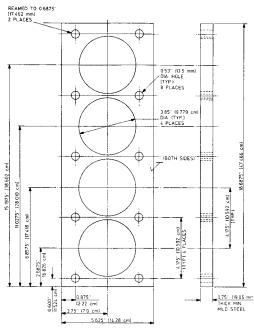
FIG. A3.36 Cylinder Block Stress Plate
