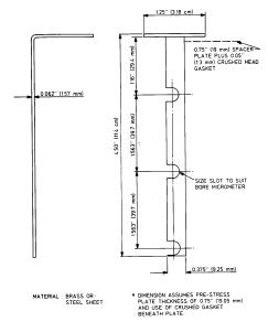
FIG. A3.38 Positioning Ladder for Bore Micrometer
