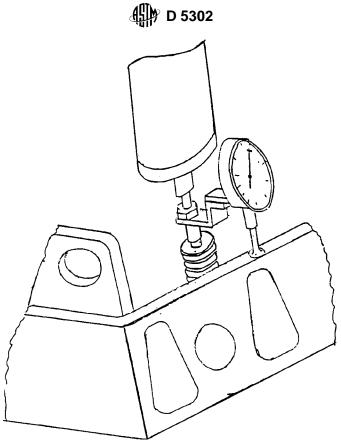
FIG. A3.46 Locating the Dial Indicator for Cylinder Head Calibration
