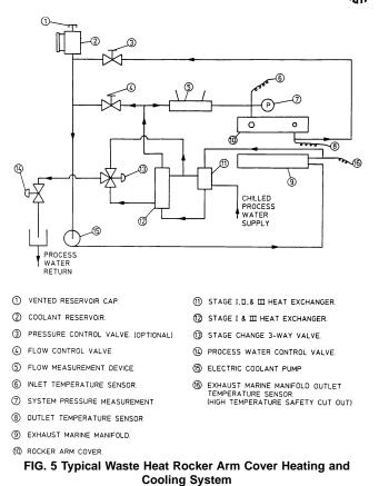
(Warning—Good engineering practices should be utilized to ensure safe operation of this system. The coolant outlet temperature of the marine manifold should be maintained below the boiling point of the coolant. High temperature, low water flow, and low water pressure alarms are recommended to prevent damage due to lack of cooling during engine operation.)
