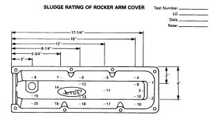
Rating sites on the top surface of the RAC are located 0.75 in. from the side or in the center.
