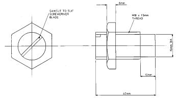
FIG. A3.29 Oil Pressure Relief Valve Adjuster
