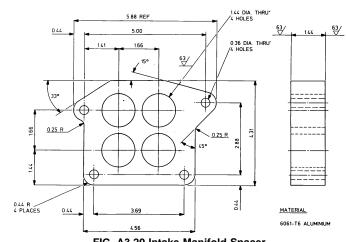
FIG. A3.20 Intake Manifold Spacer
