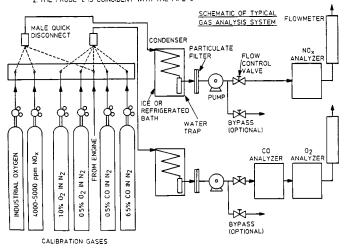
FIG. 3 Exhaust System and Exhaust Gas Analysis Apparatus
