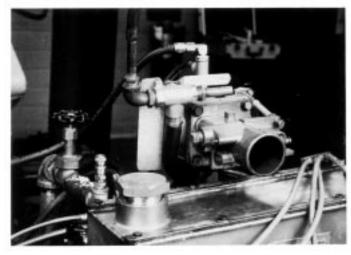
FIG. A3.18 Engine Ventilation System, Three-Way Valve
