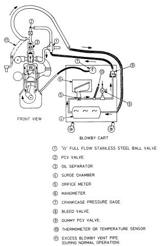
FIG. 7 Blowby Measurement Apparatus
