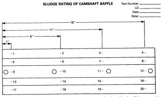
All rating sites are located according to the dimensions shown and at the midpoint of the appropriate plane.
