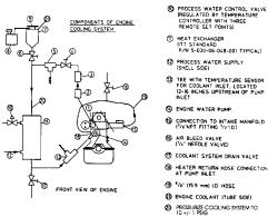
Note 1—Observe temperature sensor locations in thermostat housing and at water pump inlet.
