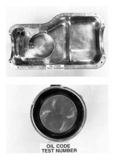
FIG. A7.15 Oil Pan and Oil Screen Photographs
