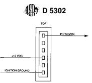
FIG. A3.43 Schematic Diagram of Ignition Module Connector
