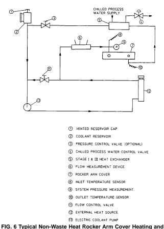
FIG. 6 Typical Non-Waste Heat Rocker Arm Cover Heating and Cooling System
