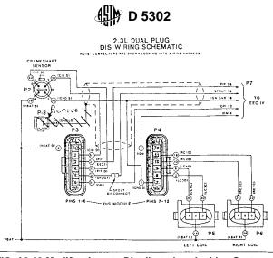
FIG. A3.48 Modifications to Distributorless Ignition System Wiring Harness
