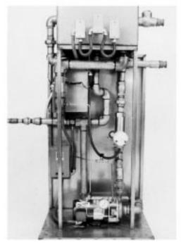
FIG. A3.41 Engine Cooling System Flushing Cart
