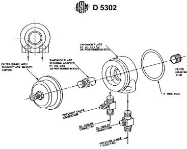
FIG. A3.39 Modified Oil Filter Sandwich Plate With Dummy Filter
