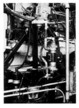
FIG. A3.11 Oil Cooling System Required Heat Exchanger Mounting, Remote Oil Filter Mounting and Typical Hoses and Fittings
