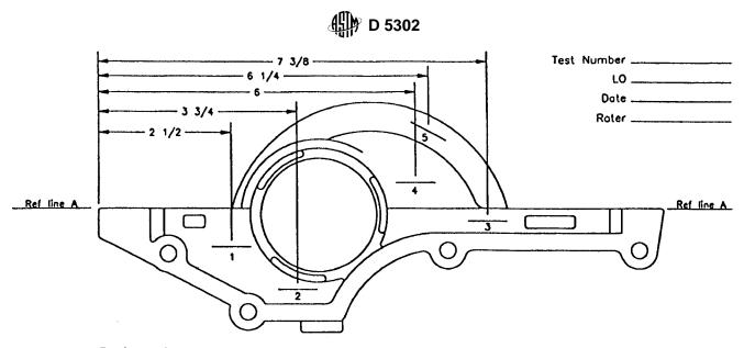
Rating site 1 is located 0.75 in. below Reference Line A. Rating site 2 is located 1.5 in. below Reference Line A. Rating site 3 is located 0.25 in. below Reference Line A. Rating site 4 is located 0.5 in. above Reference Line A. Rating site 5 is located 1.5 in. above Reference Line A. The depth gauge should be oriented as indicated by the (-----) and the dimensions shown on the drawing.
