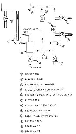
FIG. 2 Schematic of Typical Engine Cooling System Flushing Cart
